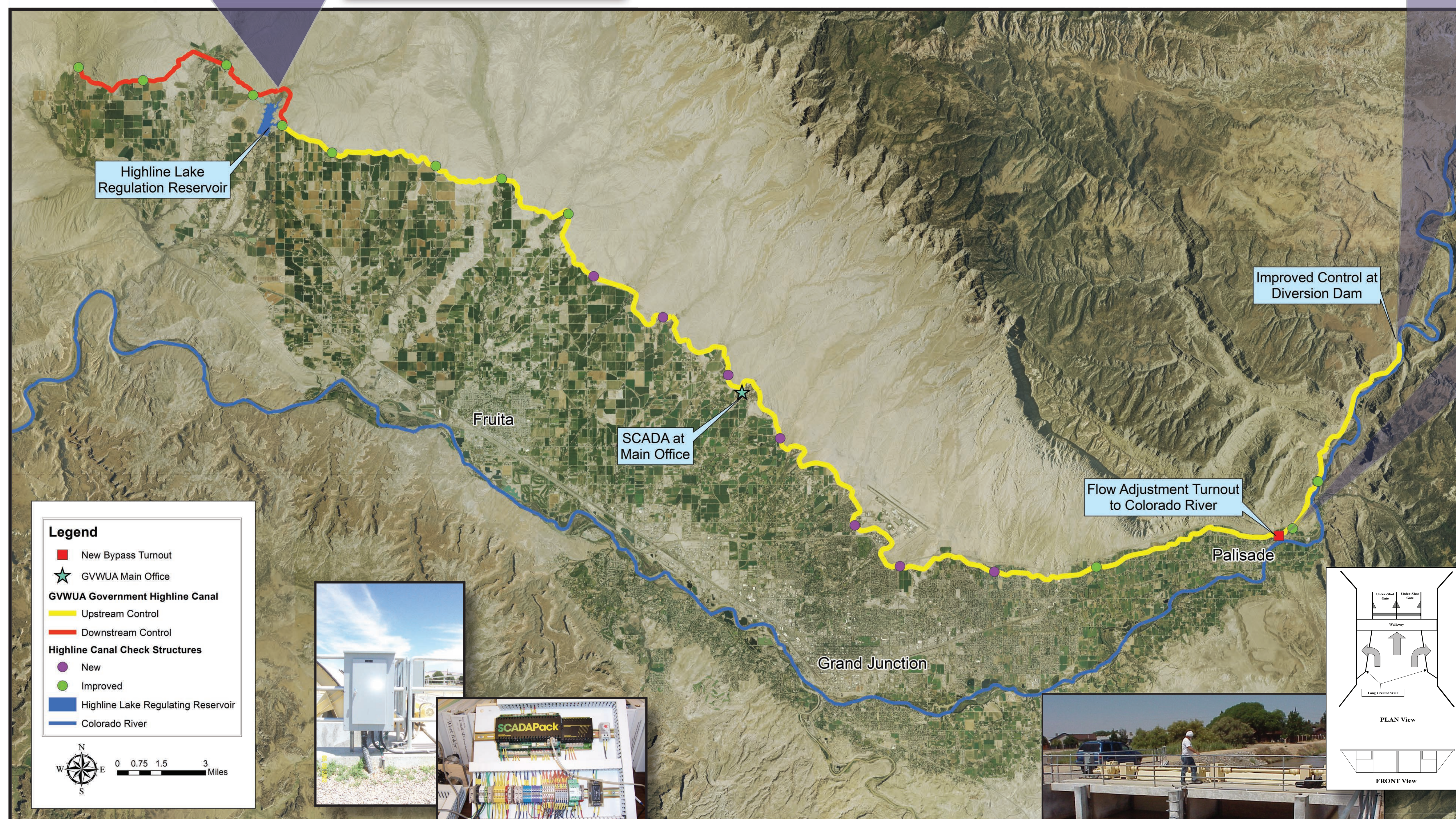
SCADA monitoring and control sites communicate with office
